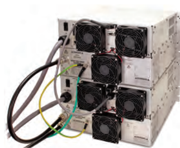
Rear panel showing connections for parallel operation
