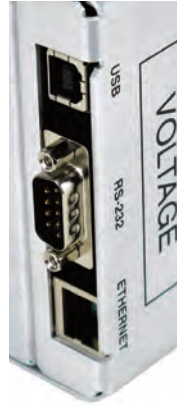
Closeup showing digital interface connectors
