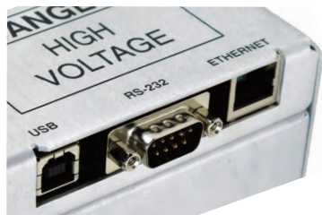
Closeup showing digital interface connectors
